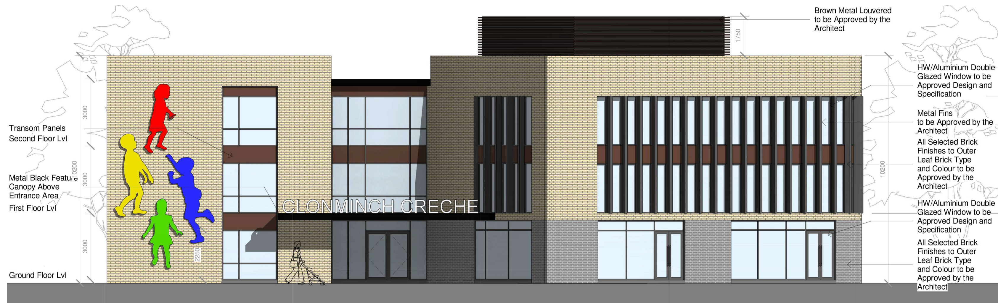
1 CRECHE-Front Elevation (East) 1 : 100
