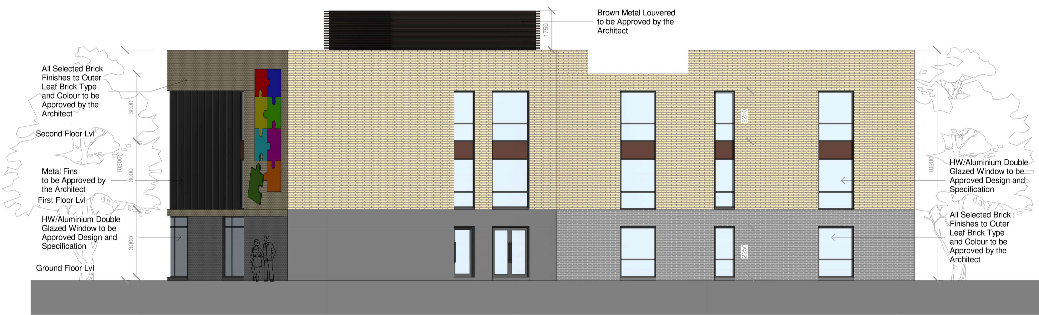
3 CRECHE-Rear Elevation (West) 1 : 100
